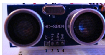
1-Vcc +5V 2-Trig 3-Echo 4-GND-masa
