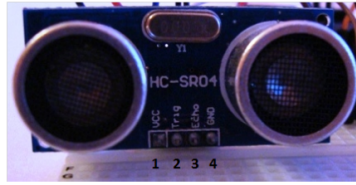
1-Vcc +5V 2-Trig 3-Echo 4-GND-masa
