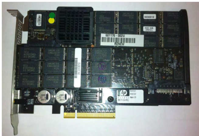
Rys. 5.3. Karta Fusion-io ioDrive DUO 640GB MLC.
