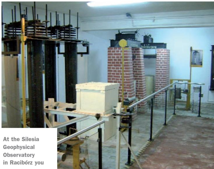
At the Silesia Geophysical Observatory in Racibórz you can see instruments for measuring and recording earthquakes constructed nearly 100 years ago
