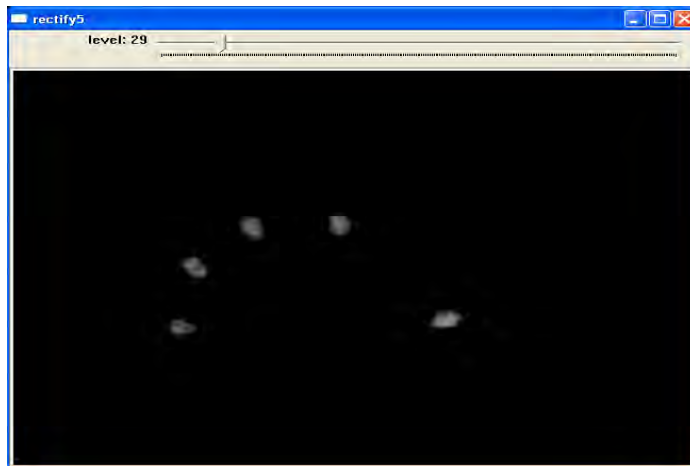
Figure 6. Reading the hand position by the infrared camera. [2]
