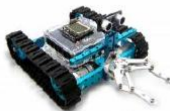
Mobile tracked platform built with the Trobot M-system kit
